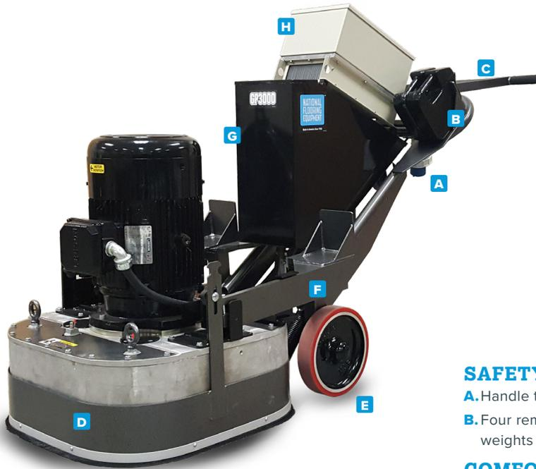
The GP3000 grinder and polisher is ideal for prepping concrete floors for topical coatings, overlays, and adhesive while also providing the variety of tooling and power needed to deliver a beautifully polished floor. The 28-inch cleaning path and increased grinding head pressure makes this an ideal machine for commercial and industrial projects.
