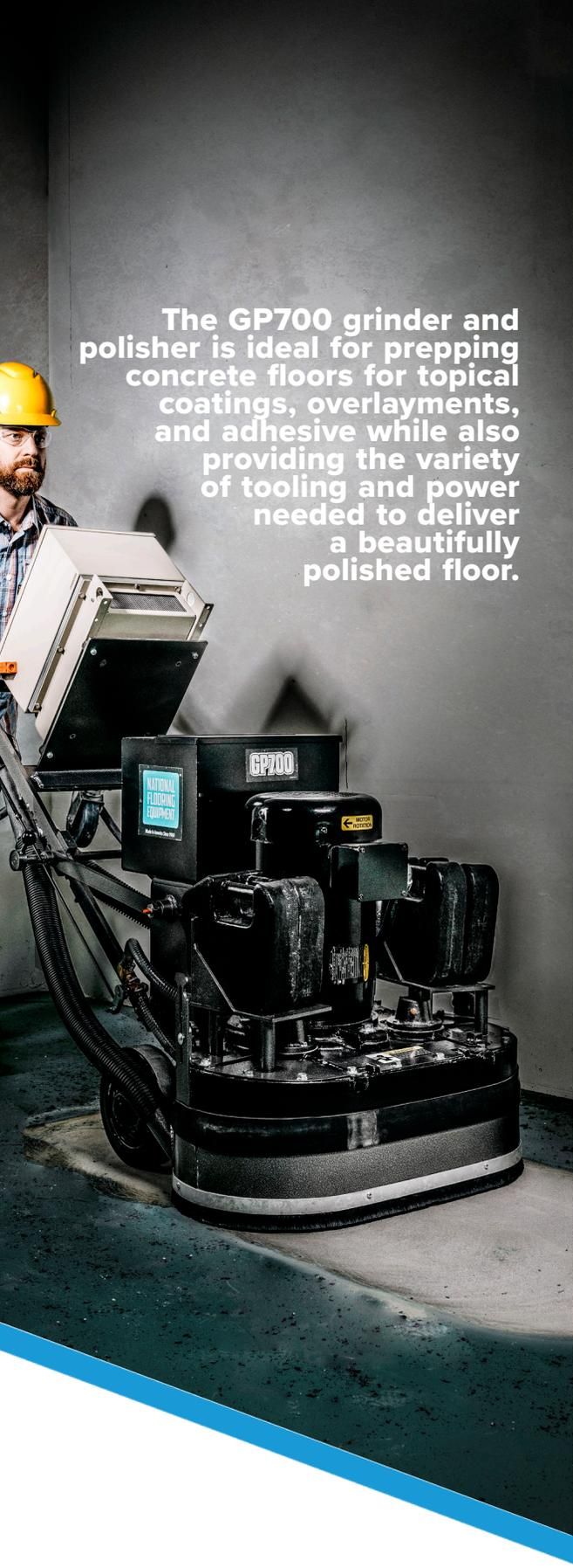
The GP700 grinder and polisher is ideal for prepping concrete floors for topical coatings, overlayments, and adhesive while also providing the variety of tooling and power needed to deliver a beautifully polished floor.
